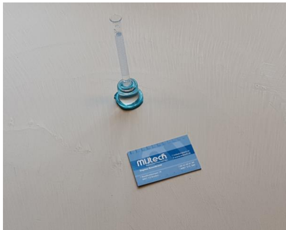
Karsten water absorption tester
